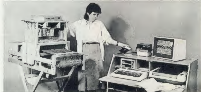
Harris Designer Loom station includes a 16 shaft 15in loom and BBC micro
